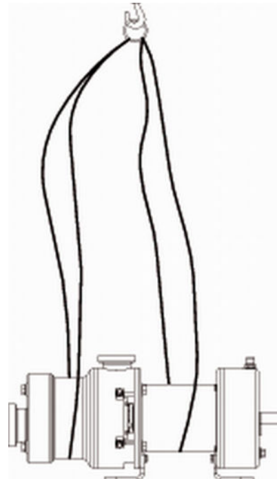
Fig. 5: Fastening the lifting tackle to the pump
