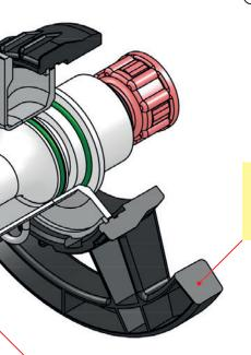
The Lutz hand wheel connects motor and pump and allows a quick disconnection
